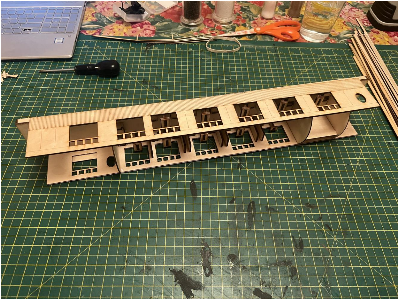
If you're assembling the kitchen coach, the large undetailed section is the kitchen area which goes at the end with the smaller window.
