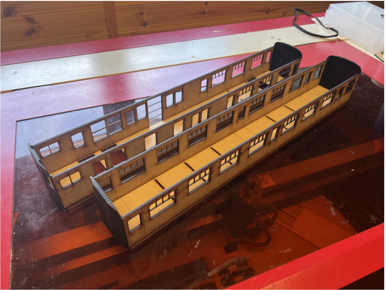
Now, glue the body together. The sides do slot inside the end panels in a slot and tab construction.
