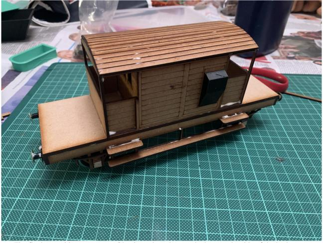
The final assembly comes now. Glue into place the two duckets on the side of the brake van. Coupling wise, these are installed by sliding the coupling hook though the buffer beam and then pinning the spring in place using a split pin (which is supplied with the couplings). The final stages of the buffers is to glue in the Brass Pins into place to form the buffer unit. Some straightening of the buffers maybe required due to their manufacturing.
