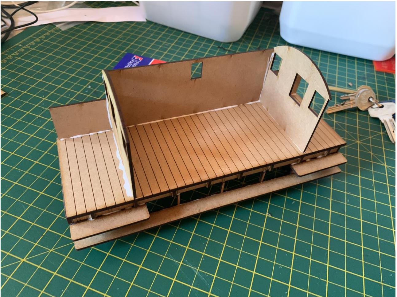
LBSCR/LSWR - To start construction of the body, glue the two internal partitions as well as one of the side pieces
