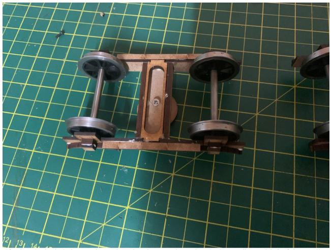
If using the included mounting point, glue that together using the larger disc and 2-3 of the smaller discs depending on your use case in a top hat shape. Then screw the bogie into the top of that top hat so the large disc is at the bottom. You can then mount that onto your model in the required place.
