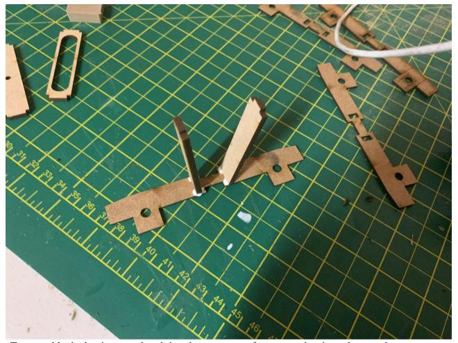
To assemble the bogies, start by gluing the two center frame stretches into place on the cut outs on the bogie side.
