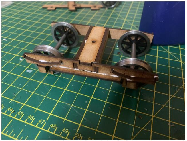
Now glue on the foot step of the bogie onto the outside. Once dry, the bogies will now form a rigid structure for running. Also glue on the axlebox covers onto the outside of each axlebox.
