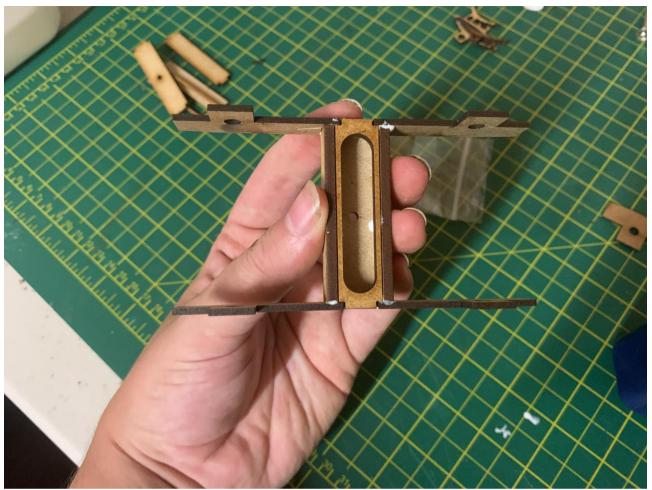
Then, glue in the bottom piece into the bottom slot.
