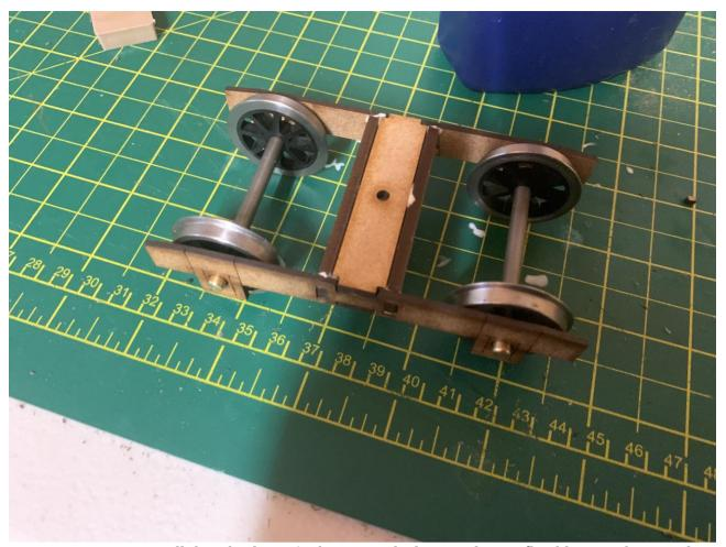
Next, its time to install the wheelsets. At this point, the bogie sides are flexible enough to gently bend to fit the wheelsets into place.
