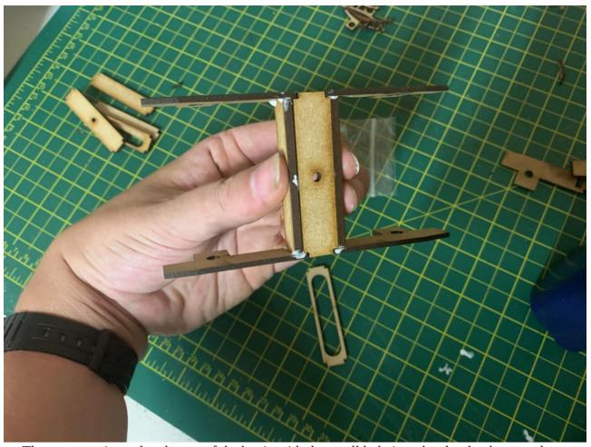
The next step is to glue the top of the bogie with the small hole into the slot that has now been created on the top of the bogie.
