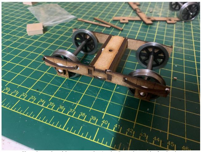
Now, glue on the axlebox outers and spring detail onto the outside of each axle.
