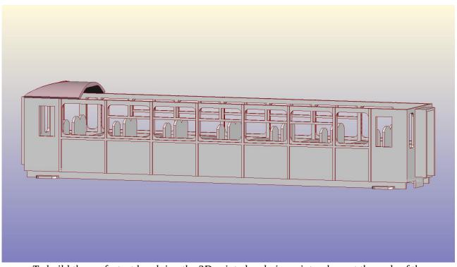
To build the roof, start by gluing the 3D printed end pieces into place at the ends of the coaches.
