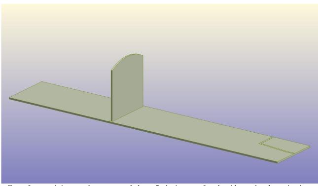
For reference, it is strongly recommended you fit the interor after the sides and ends are in place due to space restraints. To assemble the interior, start by gluing the central partition into place over the etched line on the floor plate.
