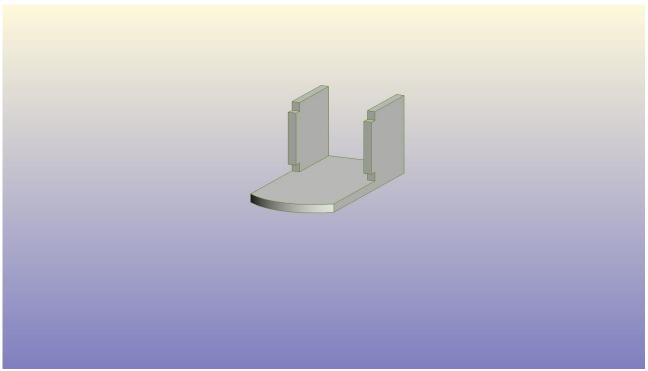
To assemble the loose chairs, glue the two seat supports onto a chair support.....
