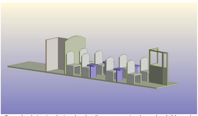
To complete the interior, glue into place the toilet compartment into the guards end of the coach.
