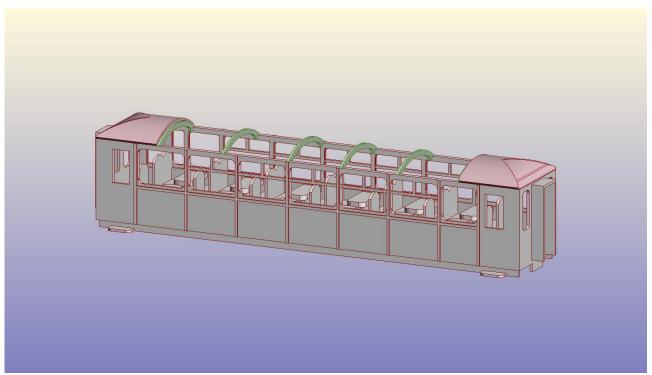
Before installing the roof, a small number of roof supports need to be glued into place. Where you place these is your choice but we recommend placing them equally along the roof.
