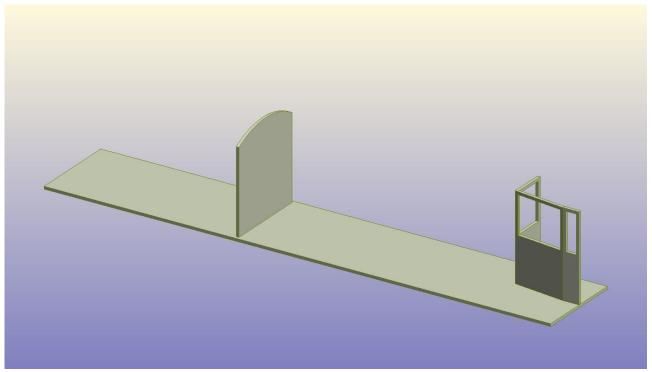
Next, install the driving compartment into its space on the floor as marked out using the etched lines.
