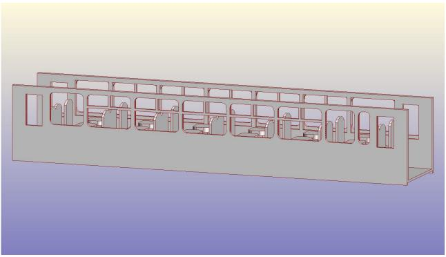
Then glue over the top, the outer layers. These can also be distinguished by having the etched detail for the beading on them.
