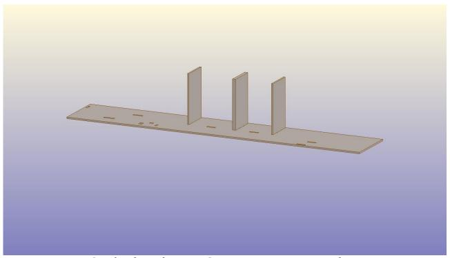
Start by gluing the centre Compartment partitions into place.
