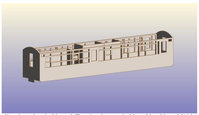
Now, glue on the ends of the coach. These sit on the very ends of the models and the top left/right hand corners will line up with the corners on the body sides.
