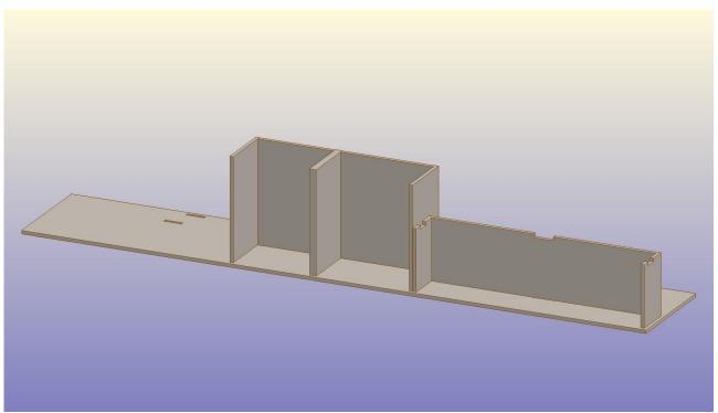
Next, start on the long counter by gluing the uprights into place making sure you get the tabs the correct way round for the top. If in doubt, do a dry run to ensure it will all slot together correctly.
