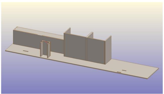
Next, start on the small counter by gluing the uprights into place making sure you get the tabs the correct way round for the top. If in doubt, do a dry run to ensure it will all slot together correctly.
