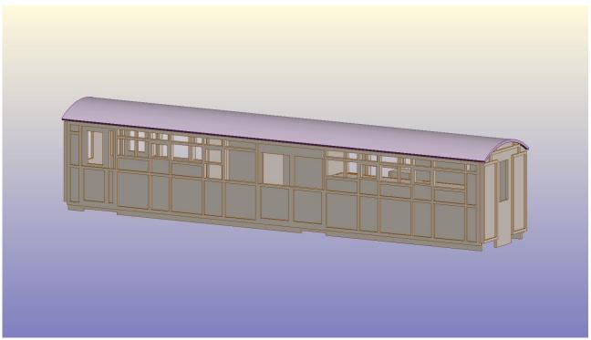
The roof itself is formed of long thin planks of wood which overlap the ends of the coach to cover the entire coach including beading. To cover the roof, we recommend either craft paper, a old shirt/sheet or masking tape all of which once painted give the perfect effect of canvas as well as smoothening the roof's curve.
