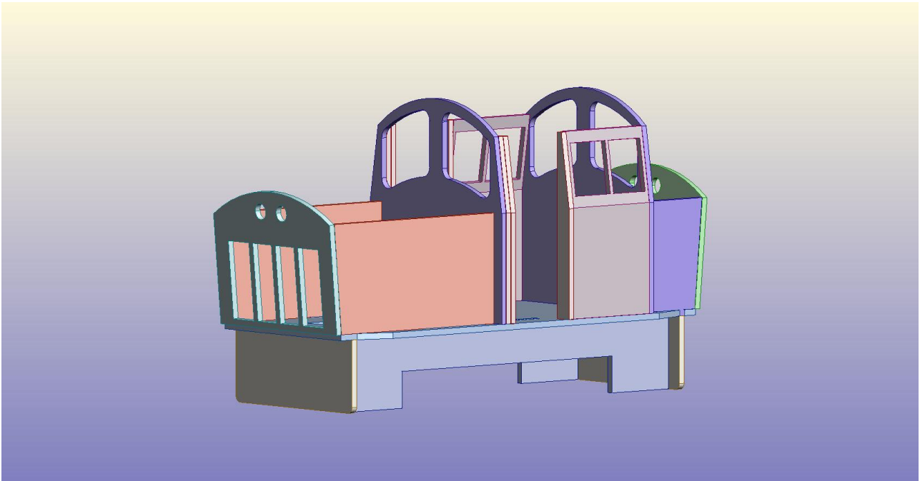
Now glue on the final cab section. This also forms the cab door inset.
