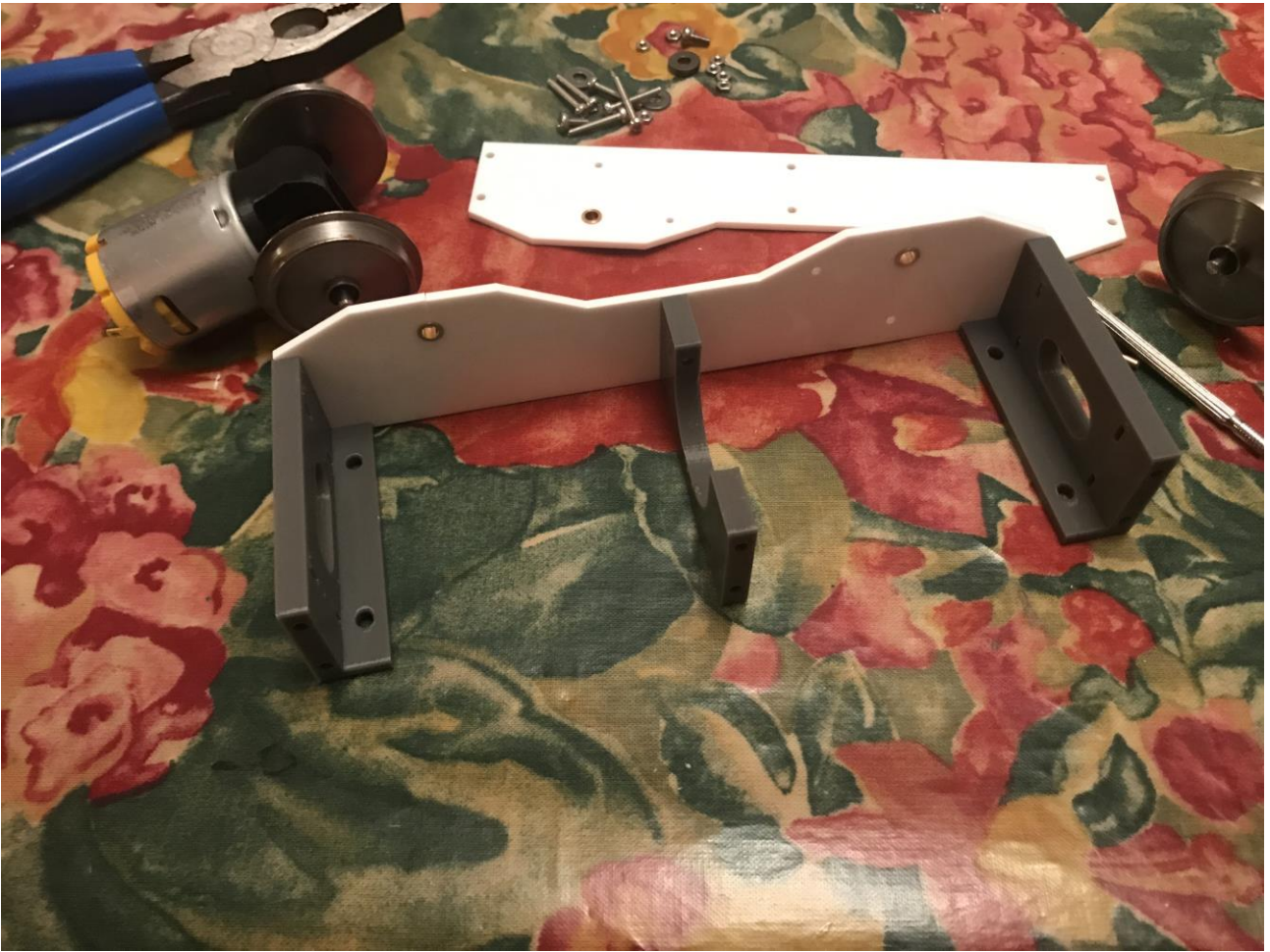
All 3 spacers shown on the chassis.
