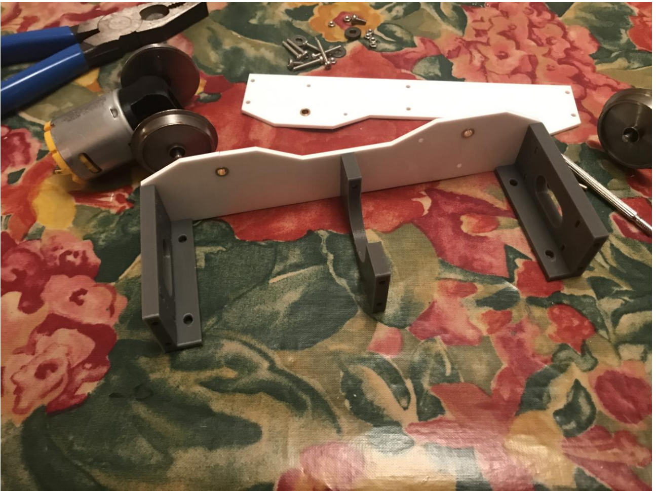
All 3 spacers shown on the chassis.
