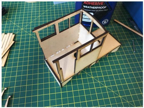
Now its time to start assemble. Glue the front and sides onto the body. The back of the sides sit level with the back of the bufferbeams.
