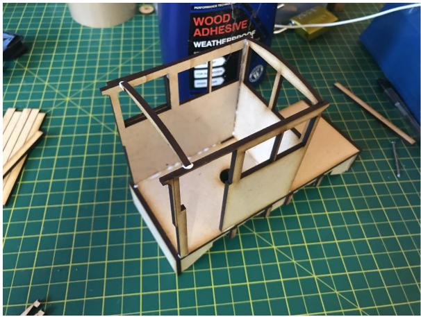
Now is the best time to glue the roof supports in. As the back of the cab is the access to the batteries, these help keep the cab in line. The hole in the floor goes inside the cab.
