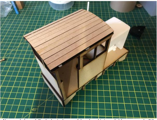
Now attach the roof. Don't glue in the rear of the cab as this is needed for access to the RC and batteries.
