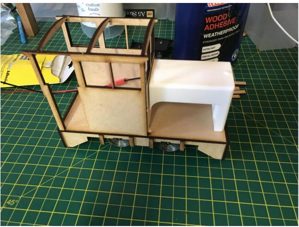
Now is the best time to attach the chassis. We recommend using 2 of the provided spacers to ensure the loco will clear the railhead when running.
