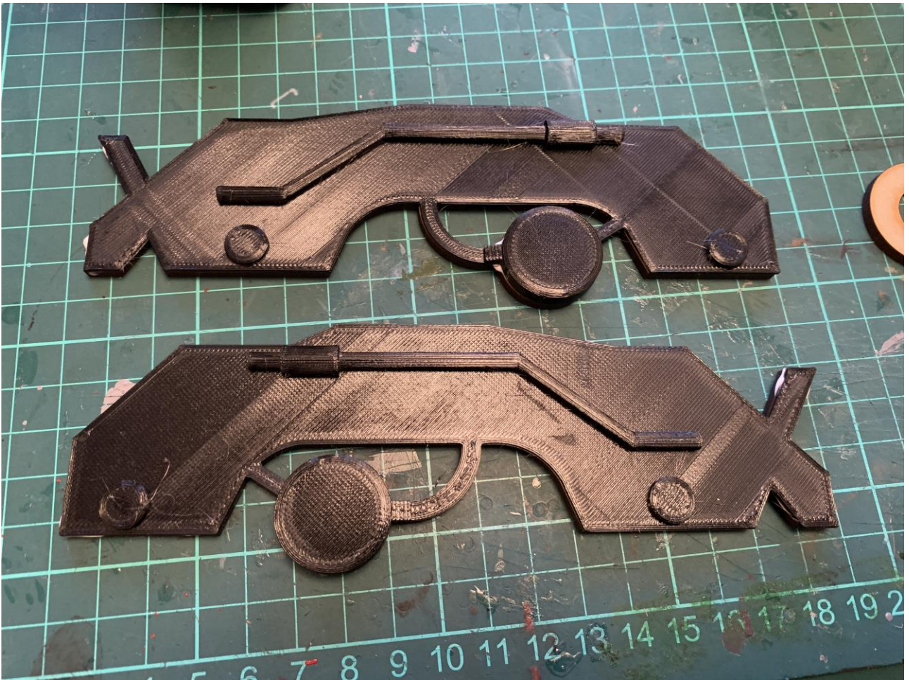
Now is a good time to assemble the bogie sides. There are two 3D printed parts that overlay the wooden substructure.
