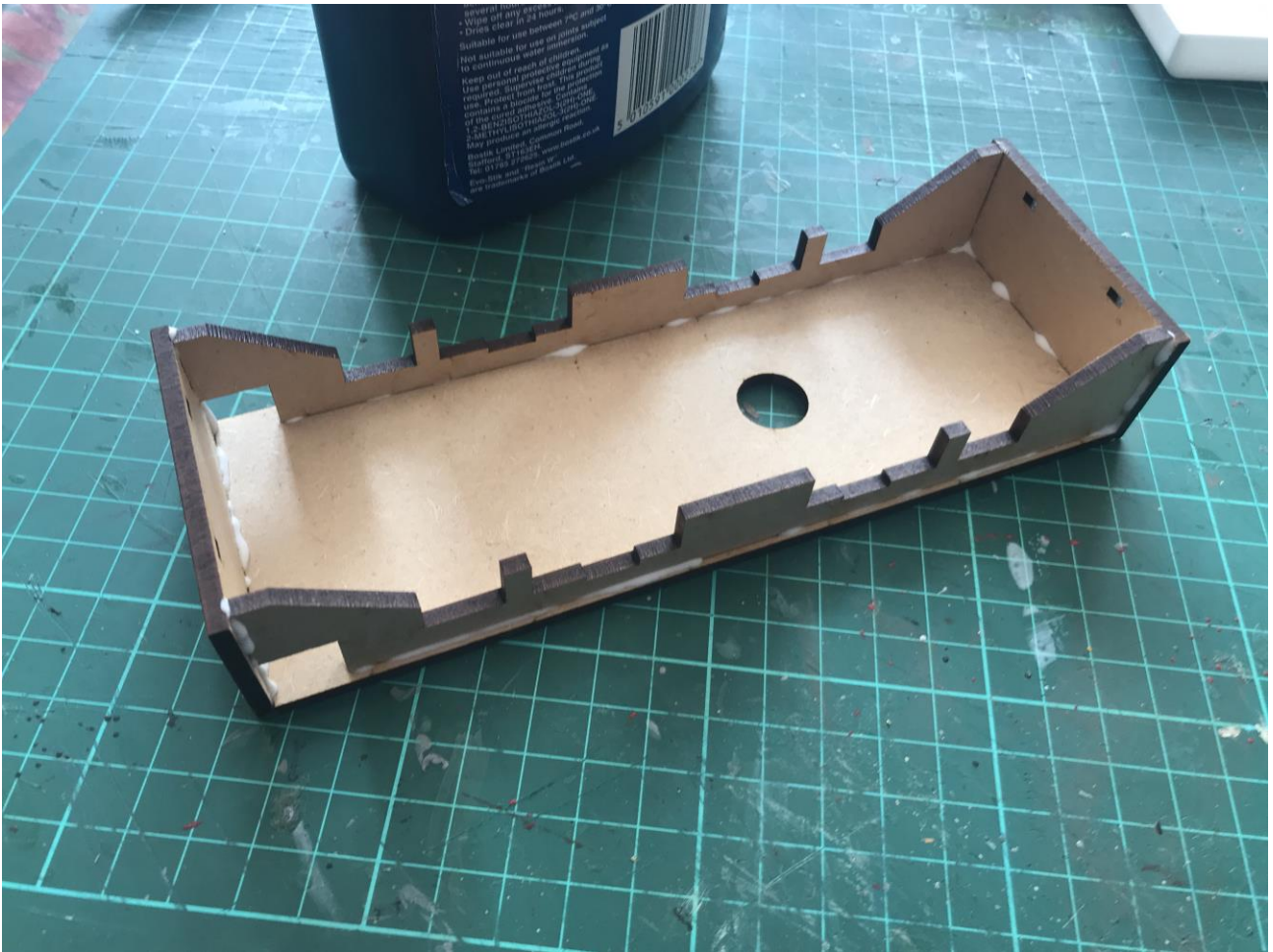
Now, glue on the buffer beams. The cut outs in the bottom of the buffer beams go at the bottom.
