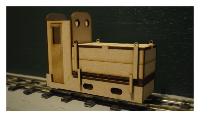
Now it is time to attach the roof. Using a piece of card, bend it around the roof shape and glue. At this stage, we recommend installing the chassis, wiring and couplings. This is down to the end user as it will vary from installation to installation. We used the switch included with the kit plus another to change direction. A slot has been left in the back of the cab for the one that comes in the chassis kit for use as a on off switch.
