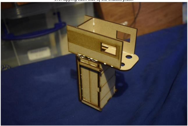
Now glue on the sides. The sides have a notch that will sit underneath the cab front giving a flat finish at the back.
