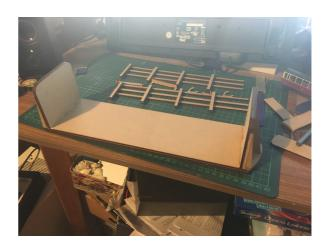
2. The First side can be now fitted and glued to the chassis. The sides sit level with the bottom of the chassis and glue onto the inside of the headstock.
