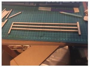
1. Starting with the sides, using the two steps, align the side strips so they are square and all aligned.
