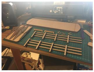
1. The headstocks can be glued on at this point making sure the rear of the headstock sits on the etched line in the top chassis plate.
