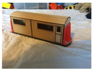
2. The two headstocks can be glued into place on the ends of the wagon so they are flush with the ends of the coach body. For assembly notes, see part 4.
