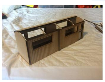
8. The Roof can then be attached at this point. The separate lengths of wood are glued onto the supports so that the complete roof is covered leaving no gaps. Once the wood has dried, you can glue a piece of Craftpaper on top of the roof to form a covering to seal any gaps. This can then be cut down to provide a neat finish around the edge.
