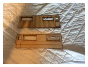
1. Starting with the sides, glue the two separate parts of the sides together with the etched detailing facing outwards. This should give a two layer side piece. There are two of these sides per Coach. The BMC-001 kit has two different sides with the BMC-002 and BMC-003 having two identical sides.
