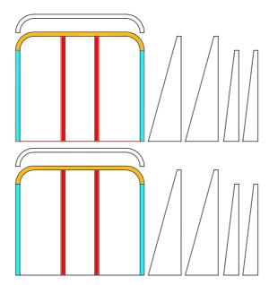
2. The two larger headstocks fit onto the centre slots in the middle (coloured red) with the two smaller ones (coloured blue). The rounded section at the top is then attached (coloured orange).
