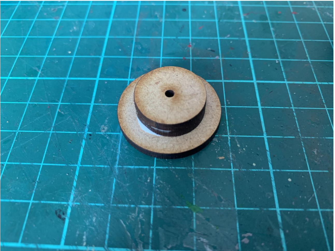
The bogie bolster is formed of 2-3 small disks and a larger disk which is mounted onto the bottom of the rolling stock you are fitting the bogies too.
