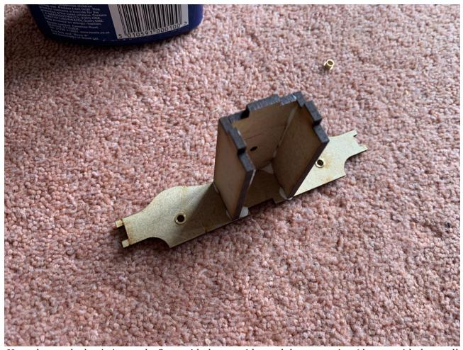
Now glue on the bogie internals. Start with the two sides and the top section (the one with the small hole).
