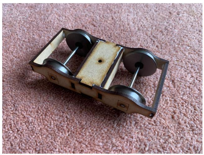
Now glue on the axle boxes. These sit on the outsides of the bogies over the etched marks on the bogie.
