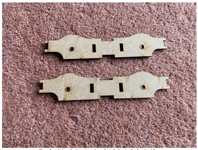
Start by gluing the bearings into their holes in the bogie sides.
