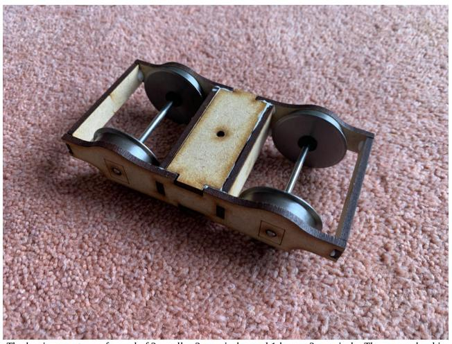
The bogie mounts are formed of 3 smaller 3mm circles and 1 larger 3mm circle. These are glued in a top hat style. These are then attached using the supplied screw and are ready for attaching to the coach.
