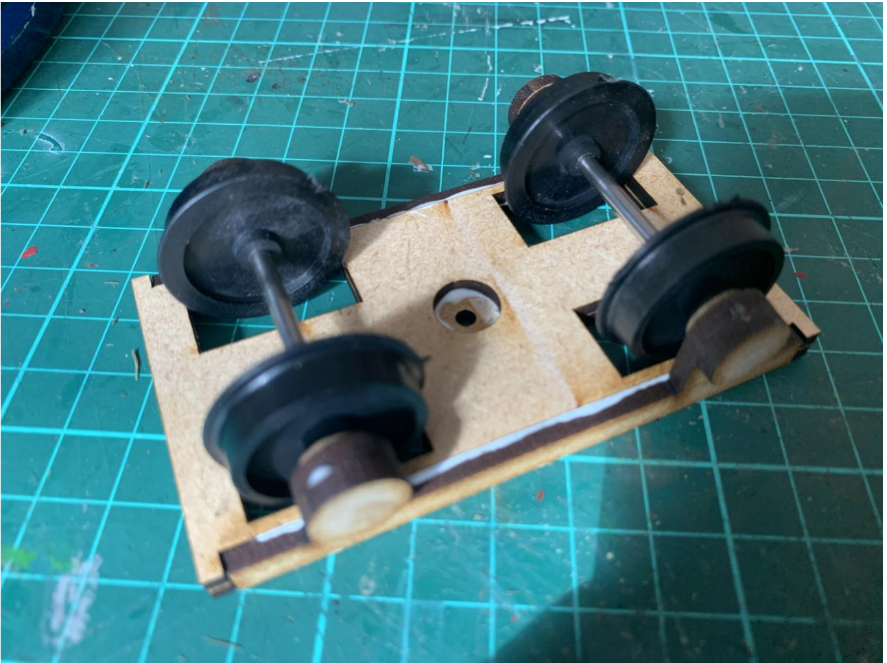
To carry out the bulk of the assembly, glue the sides onto the sides of the base plate inserting the wheels at the same time.
