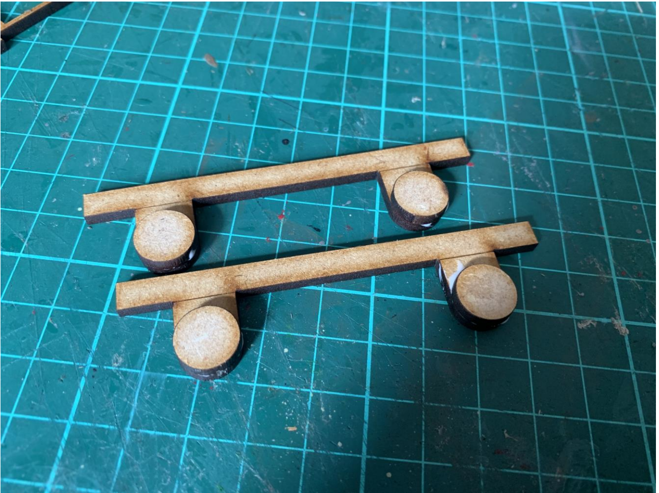
The sides of the bogies are the next thing to be assembled. The outer axlebox covers are glued onto the outside of the sides.
