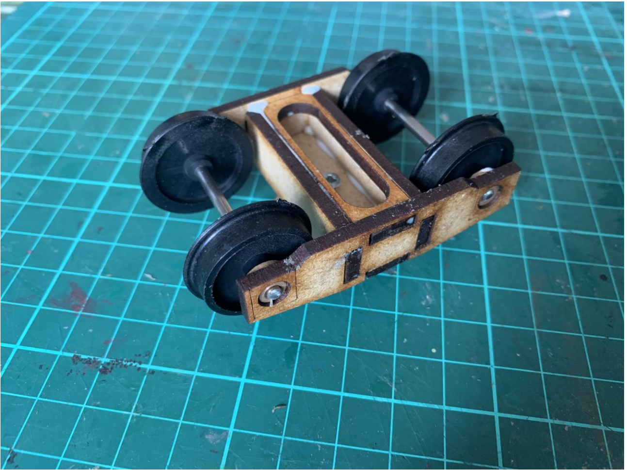
Next, glue on the second bogie side along with the wheelsets to complete the core construction.
