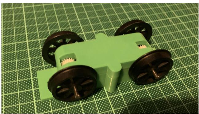
Now slot the bottom piece onto the chassis unit. To test the unit, apply power to the motor while holding the unit together to ensure the wheels turn correctly. Once its been confirmed all is well, the card piece and chassis halves can be glued together ready for running in. It is recommended you run the chassis for 30 minutes in each direction for your first running in. The chassis will run smoother the more it is run.
