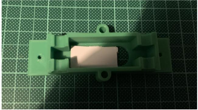
The Motor can be installed next. Use a thin piece of card placed on the top of the motor housing to gently press the motor into place. We don't recommend gluing it in place until the gear mesh has been checked and it runs freely. Then you can glue it in place. The way you can tell the gearing is correct is the wheels will not turn when the chassis is held together.
