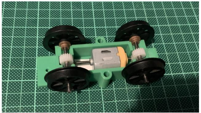
Now insert the axles into place making sure the bearings sit in the notches on the bearing sides.
