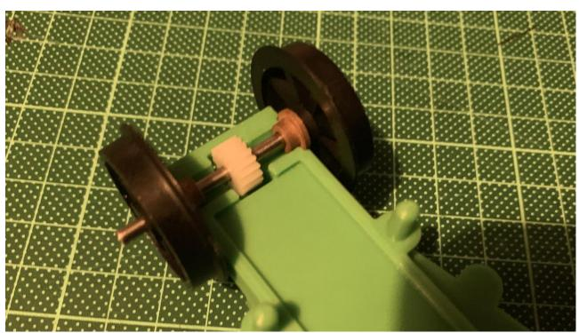
Next assemble the axles. They are formed of 2 wheels, two bearings and two spacers (45mm gauge only) which slide into place. We recommend using Loctite to fix the wheels in place using the back to back of the supplied parts. The assembly for 32mm gauge is: Wheel, Bearing, Gear, Bearing, Wheel. The assembly for 45mm gauge is Wheel, spacer, bearing, gear, bearing, spacer, wheel. The spacer is a small cylinder with a hole though the middle of it.
