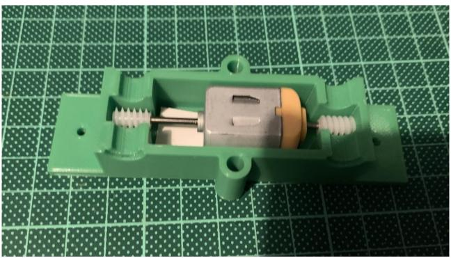
The motor then slots into the slot with the electrical tabs at the end with the large hole in which will be the top when assembled.
