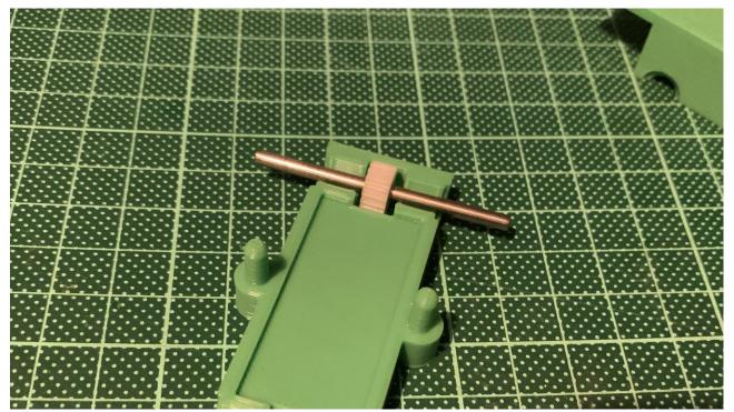
Start by sliding the gears onto the axles. These are a tight fit and will require a little force to slide in place. We recommend using the chassis block to ensure it is in the middle of the axle.
