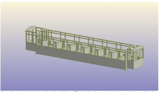
Now glue into place the coach ends and doors. The double doors go into place with the smaller door closest to the passenger compartment.
