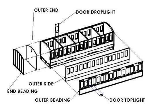
The Outer Beading is added next, ensuring the ends line up with the Outer Sides and the top edge flush with the Outer Side. Once they are dry the End Beadings are fitted the edges are flush with the Outer Beading and the roof profiles matches.
