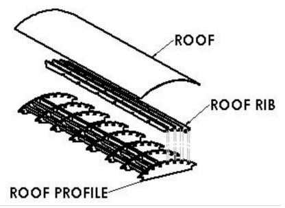
sandpaper wrapped around a piece of timber. Work gently on the edges of the roof profiles along the length of the roof structure, sanding a number of profiles at the same time to get a straight edge. Once a good, snug fit has been achieved the end Profiles can be glued to the Roof Ribs, and refitted into the body assembly. The cling film acts as a barrier between the roof and body to stop the 2 being glued together.
