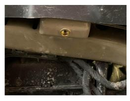
Install the riv nut at existing thru hole, on left and right side forward upper support bracket (Driver side shown)
