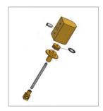
As noted above the cylinder assembly is factory lubricated and assembled to exacting standards and it is recommended that local inspection should not be undertaken. Please note that a stuffing gland has been added to reduce steam leakage past the connecting rod. This can be seen in the image on the cover page.
