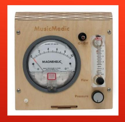
CHECKING FOR LEAKS: MAG MACHINE
