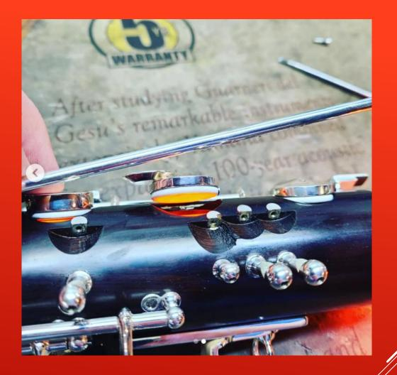
CHECKING FOR LEAKS: LEAK LIGHT
