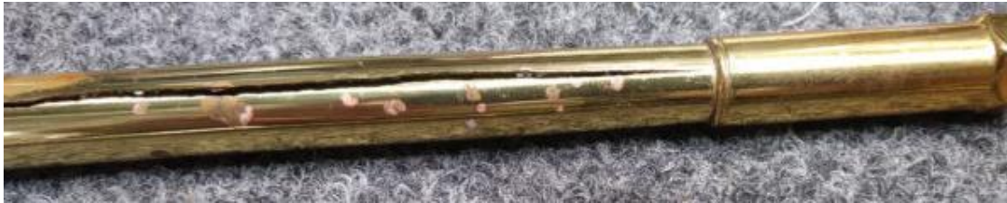
Red rot on a lacquered leadpipe www.mencheymusic.com/case-yearly-brass-tune-up
