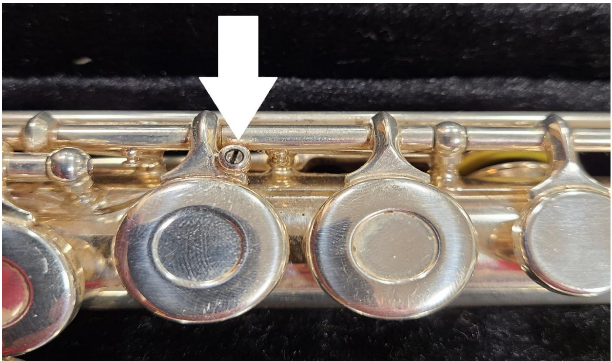
Left hand adjustment screw on Gemeinhardt- easy to find! Truly putting the "gem" in Gemeinhardt.
