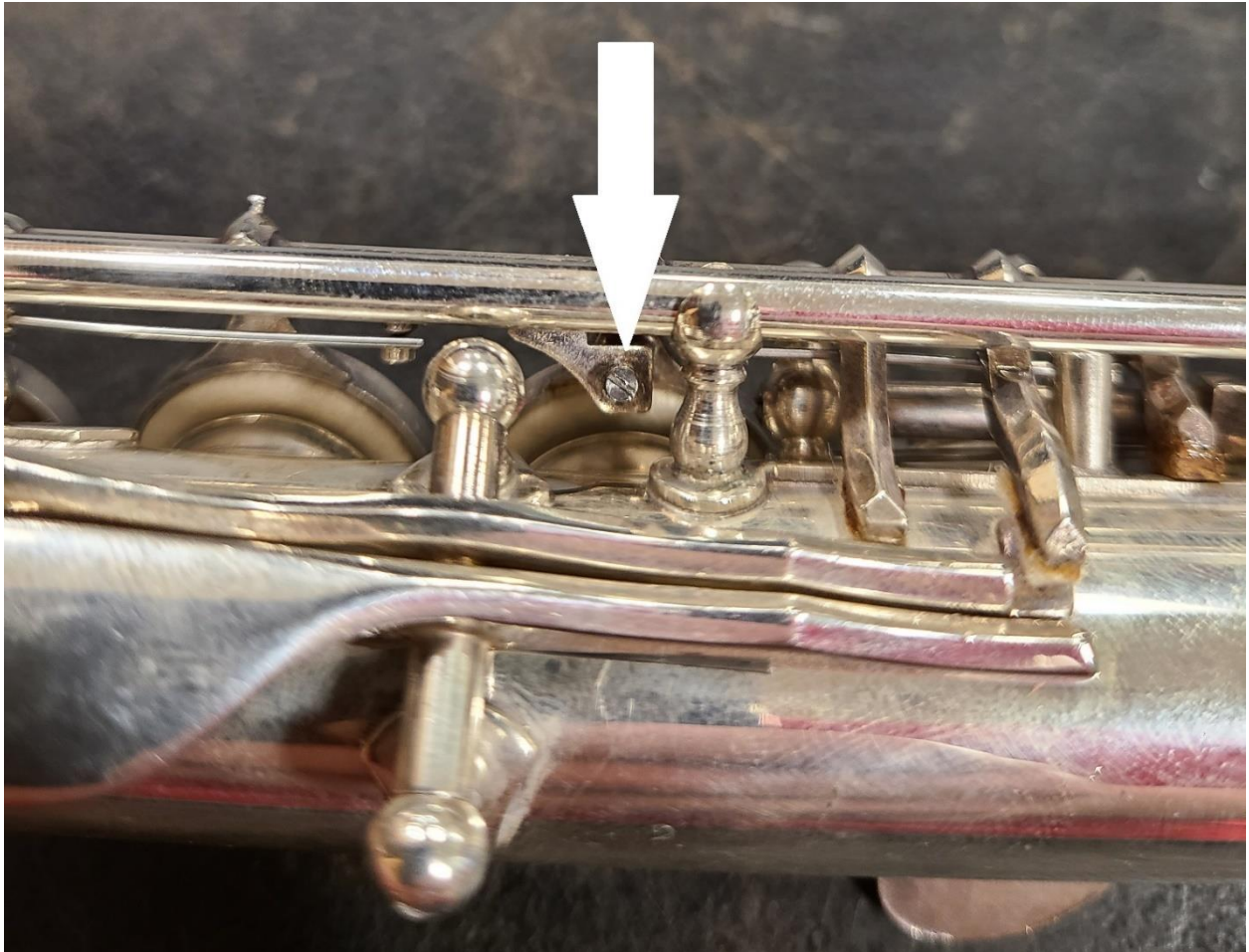
Left hand adjustment screw on Yamaha- hidden in back and obscured by thumb key! 😊
