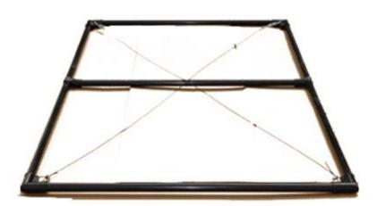
Measure the distance between one opposite pair of corners and then the other pair. If these distances are equal the door is square. If they are not equal, tighten and/or loosen the appropriate turnbuckles to equalize the distances and make the door square. Cut any excess line about 4 inches beyond the U-bolt clamp in case there is ever need for further adjustment.
