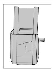
• Look for wear and damage on the bag due to use (cuts, signs of chemicals or burns, discoloration, loose tears...).
