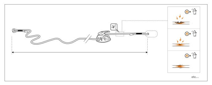
• Carry out a tactile inspection of the core along the entire length of the rope (hard spots, swelling, soft or crushed areas...).
