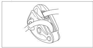
• Check the condition of the handle (marks, deformation, cracks...). Check that the handle return spring is working properly.
