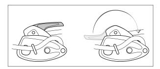
• Check the condition of the rivets (marks, deformation, cracks, corrosion...).
