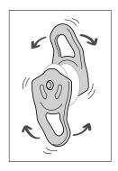
• For pulleys with moving side plates, verify that the side plates rotate properly.
