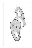
• Check the condition of the side plates (marks, deformation, cracks, corrosion, wear...).
