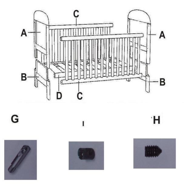
Put end frames (AB) on the floor (on soft pad or carpit to prevent scratching or damage) - screws up. Screw in long silver housings (G) in prepared metal holes. (one End frame (AB) lef for later use)
