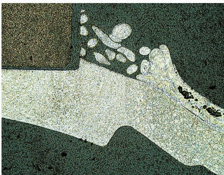
Weld structure, brightfield
