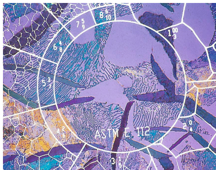
Grain sizing reticle overlay
