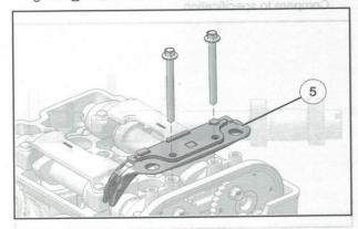
Remove the remaining two bolts that retain the front camshaft carrier (a) and carefully lift the carrier off the camshafts.
