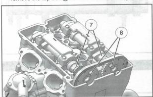
Rotate the engine to allow access to the remaining bolt on each camshaft sprocket.
