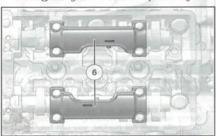
Install the Cylinder Holding & Camshaft Timing Plate (PU-50563) into the end of camshafts as shown. Use an open-end wrench to rotate camshafts slightly.
