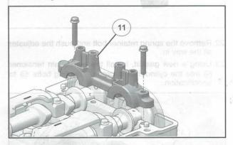
20. Install the fixed cam chain guide @ and two retaining bolts.
