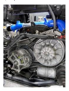
Step 7: Install clutch cover back onto the vehicle.
