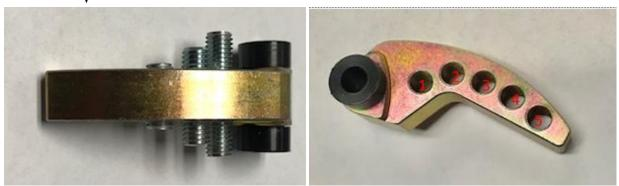
**NOTE:** Always install a set screw on both sides of the weight arm. Install the screws with the provided blue thread locking agent. Make sure the screws are installed with an equal amount of thread engagement.
