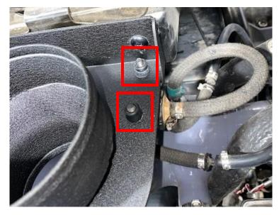
**Step 11:** Mount the XR Series air filter bracket to the OEM firewall bracket. Tighten the silicone to the turbo inlet and XR Series air filter bracket.
