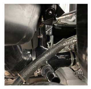
**Step 9:** Remove the (2) OEM M6 thread tabs from the plastic shroud, and place onto the bracket behind the drivers seat. See photo below.
