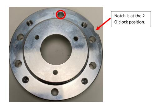
Step 5: Install the new billet PTO cover, torque all (6) M8 x 35mm Torx screws to 17 ft lbs.
