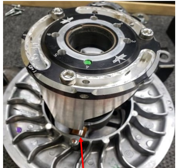
Helix must be rotated clockwise so the ramp will clear the roller.
