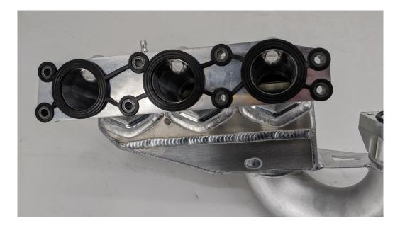
Step 12: Install the big O-ring on the side for the throttle body again use di electric grease.
