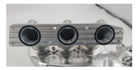
**Step 11:** Install the big O-ring on the side for the throttle body. Use di electric grease.
