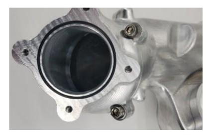
**Step 12:** Install throttle body onto the new plenum, make sure the plug is facing towards the engine and using the M6 x 1 x 45 bolts to fasten it on.
