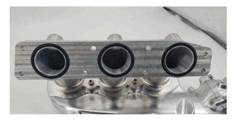
**Step 11:** Install the big O-ring on the side for the throttle body. Use di electric grease.
