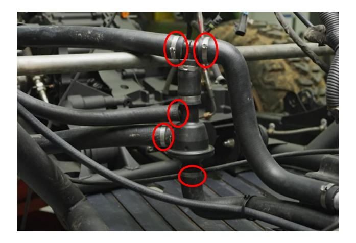
**Step 2:** Remove the hoses that you removed the pinch clamps from. Remove the thermostat housing from the vehicle.
