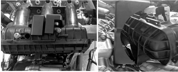
Step 7: Now that all (3) pieces are installed, start all (4) bolts before tightening them down. Put Loctite on the threads of the bolts.
