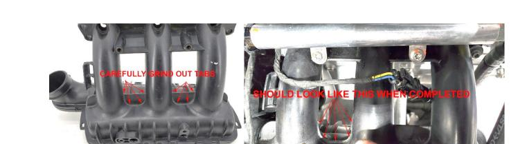
**Step 5:** Using a Dremel tool or air grinder, remove tabs shown in the picture below. Be careful not to compromise the integrity of the runners by only removing as much material as necessary for THE CLAMP
