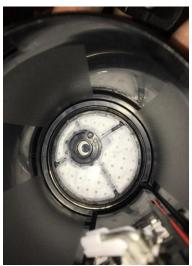
Step 9: Plug the electric connection into the pump.
