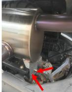
**Step 3:** Install and mount the Muffler Bypass Pipe and bracket with the bolts loosely installed then hook up all four springs. Keep the bolts loose until the rear fascia is reinstalled.
