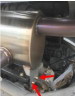
**Step 3:** Take the 02 sensor out of the exhaust. Treat the tip of the sensor gently.
