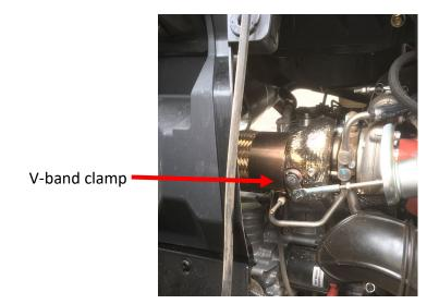
Step 6: To remove the catalytic converter, slide it toward the front of the car, over the mount. Next, swing the turbo side down until it is vertical. Finally, pivot the entire converter out of the shielding and remove from the vehicle. Follow the images below. NOTE: These images were taken without the rear cargo rack for better visual instruction, the rack can be left on when removing the converter. Motions are indicated with thick red arrows.
